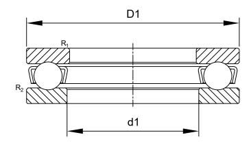
R<sub>1,2</sub>: min0.3 mm Chamfer Dimension Washer
