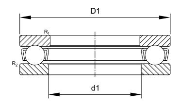
R<sub>1/2</sub>: min0.6 mm Chamfer Dimension Washer
