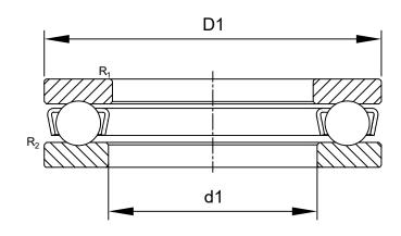
R<sub>1,2</sub>: min 5 mm Chamfer Dimension Washer
