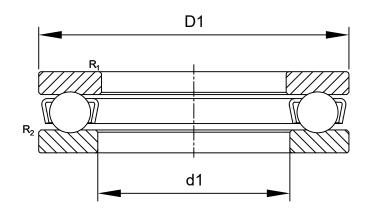
R<sub>1,2</sub>: min0.15 mm Chamfer Dimension Washer
