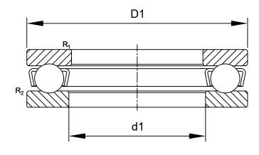
R<sub>1,2</sub>: min0.15 mm Chamfer Dimension Washer
