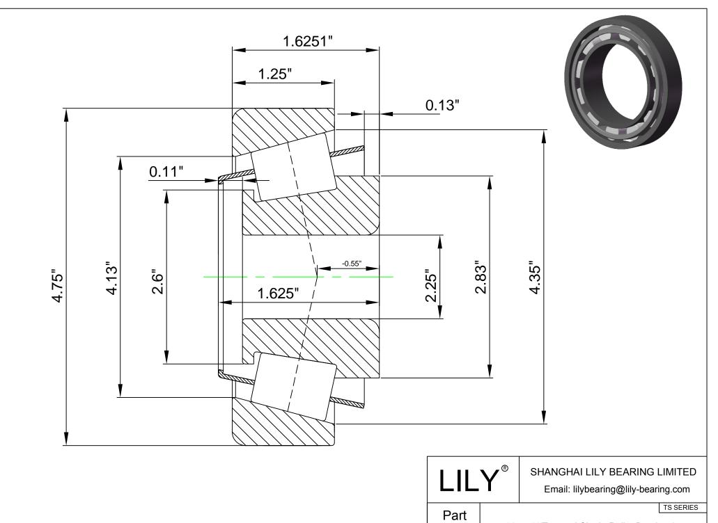
623V-612V(Tapered Single Roller Bearings)
