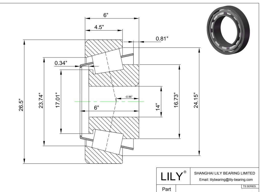
EE121140-121265(Tapered Single Roller Bearings)
