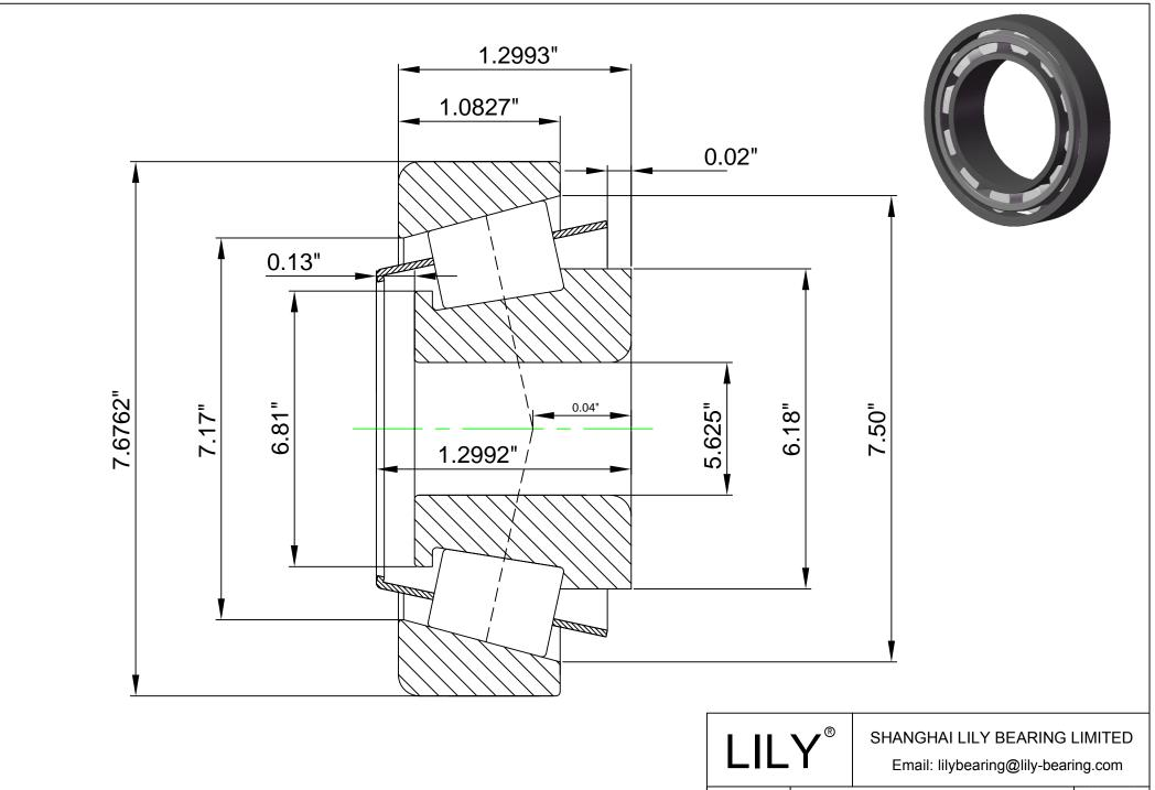
TS SERIES Part LM229147C-LM229110(Tapered Single Roller Bearings) Number
